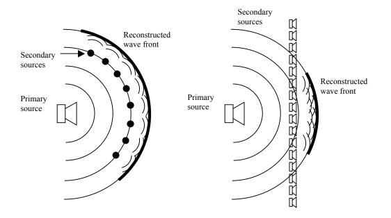
Fig. 3 – On left, the Huygens's principle of construction. On right, the principle of construction applied to sound fields reproduction by means of practical and real sources.
