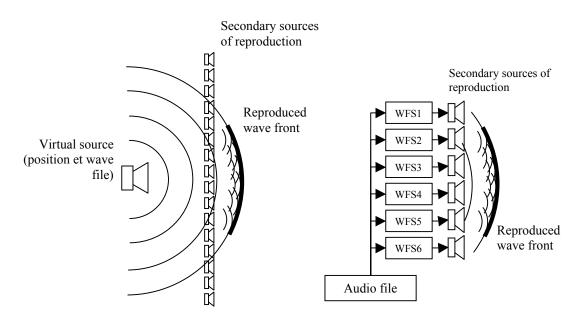
Fig. 4 – On left, the principle of construction of Huygens applied to the reproduction. On right, a simplification of the realization of WFS for a single virtual source.
