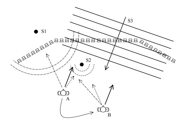
Fig. 5 – Illustration of a virtual scene formed with a spherical source S1, a spherical source focused in S2 (in front of the loudspeaker array) and from a source of plane waves S3. The listener can be in two positions (A or B) for which the perceived directions of the virtual sources are represented with arrows with graphical displays corresponding to the virtual sources.
